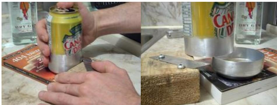
Once you have cut the two cans, it's time to assemble your stove. The Hannah Stove is press fit. If you have peace of mind, you can just align the can bottoms and fit one right into the other. It is easier to do that if you enlarge one can bottom a bit. That's what the third soda can is for. This can should still be sealed. Select the can bottom with the less
