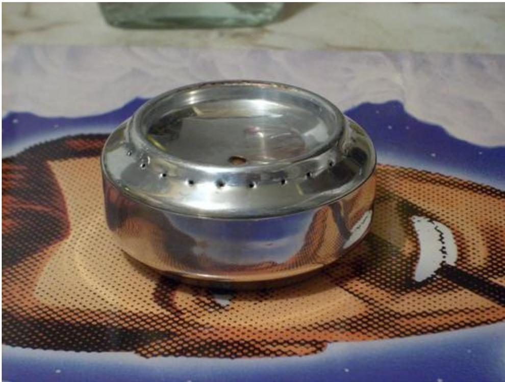
While I was experimenting with early prototypes, it became evident that I wanted a [pressure stove](#). Pressure stoves are more fuel efficient and they have fewer internal parts. I wanted something easy to build but most of all, I wanted a method that would yield consistent stoves. After learning the hard way, I decided that safety was to take precedence over those two requirements. Building a Hannah Stove will take you only one hour. Lets get started with the requirements.
